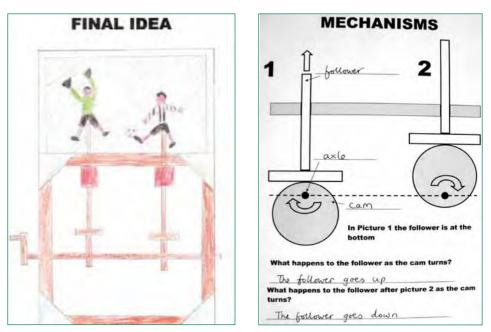
Sam constructed the frame structure upon which to mount the cam mechanism and built his cams by drilling offset holes in circular timber disks *using appropriate tools and equipment* (a characteristic of Level 4).
