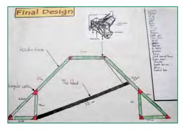
The roadway was made from thick card and raised with a motor and pulley system.
