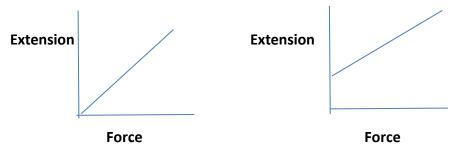
The graph on the left hand side – shows that the extension is directly proportional to the force e.g. if the force was doubled then the extension would be doubled etc The graph on the right hand side – shows that the extension is proportional to the force applied. Both show positive correlation
